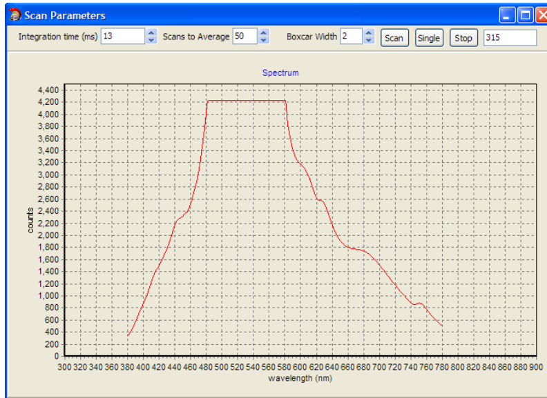
Incorrectly Adjusted Integration Time: Integration time set too high; part of spectrum is saturated
