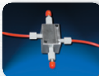
Low Volume flow cell with PTFE tubing and Upchurch fittings
