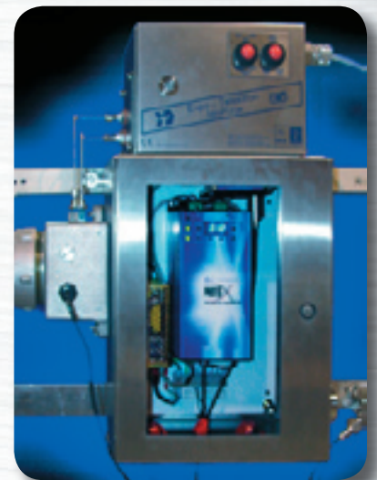
Example of a UV transmitter suited for a C1D2 area
