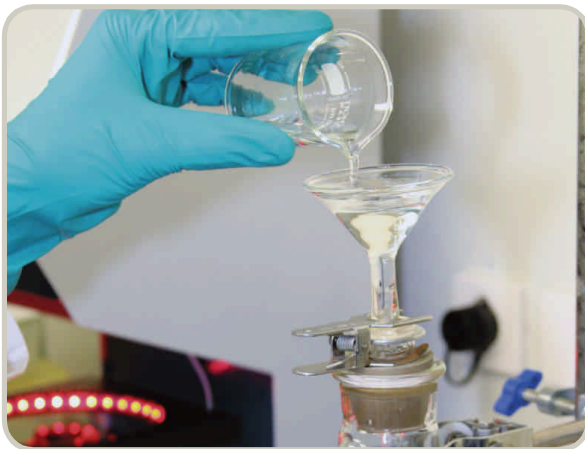
Effective Filtration Area (EFA) ø 4 mm standard; selectable ø 1 - 18 mm
